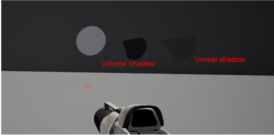
Figure 4.6: Visual comparison of Unreal shadow map shadow ( Unreal shadow ) and our shadow ( volume shadow ) with the same test setup as in Figure 4.5. We captured this screenshot with the shadow caster (cone) in motion. The shadow created by our algorithm is still sharp, while Unreal’s own shadow map shadow is blurry. This is caused by a motion blur post-processing effect, which our algorithm does not include.
