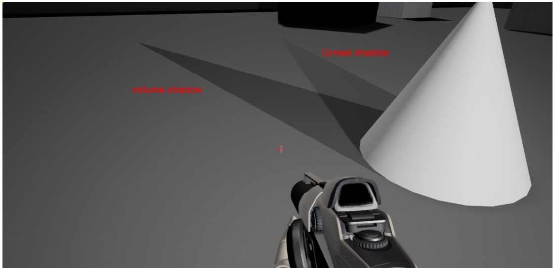
Figure 4.5: Visual comparison of Unreal's shadow map shadow ( Unreal shadow ) and our shadow ( volume shadow ). The test setup is similar to the one shown in Figure 4.3 and Figure 4.4. The sharp shadow edges created by our implementation can be observed even more prominently, especially at the pointed top of the cone's shadow.
