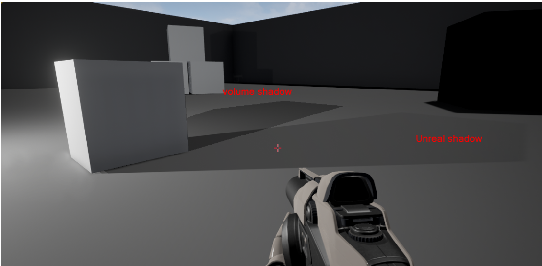
Figure 4.3: Visual comparison of Unreal's shadow map shadow ( Unreal shadow ) and our shadow ( volume shadow ). A cube is set up as the shadow caster. Two light sources are used to offset the two shadows for visual comparison. The sharp edges of our shadows and the correct summation of shadows in the overlapping area can be observed.
